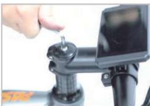
Screw on and tighten
