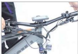
Put the handlebar on the stem
