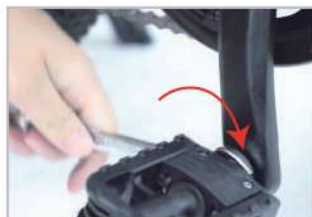
Rotate clockwise to tighten
