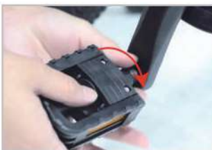
Installed on the chainwheel side crank
