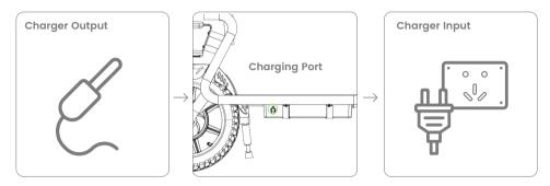
Connect the charger output to the charging port on the eBike first, then connect the charger input to the mains. Stop charging when the battery is full.
