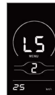
Fig. 7-2 Speed Limit Setting Interface
