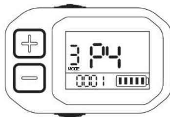
P4: setting the default speed level; 0 means starting at speed level 0, and 1 means starting at speed level 1.
