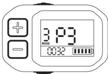
P3: setting the speed limit within 0-25km/h; The default speed limit is 25km/h.
