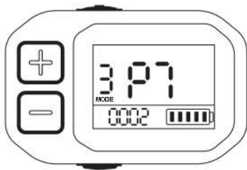
P7: turning on/off the bike locking function; 0 means the locking function is turned off, and 1 means the locking function is activated. The default setting is 0.
