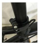
**IMPORTANT:** Do not raise the seat post above the "minimum insert" line clearly printed on the backside of the seat post. Raising the seat post above the minimum insert line can cause the seat post to fail, which could in turn result in loss of control of your GM30 and could cause you serious injury.
