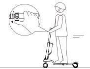
4.Continue to press the thumb shifter to speed up, turn the grip to adjust the direction.
