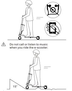
▲ Be careful of the road with roadblock, sandstone, ponding, mud, wet, ice and snow, slope (angle >15°) stairs, dark area when you are riding.
