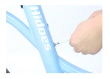
Attach the bike kettle holder to the upper tube
