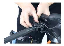
Insert the seat tube, Lock the quick release handle in the direction
