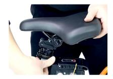
The battery is locked by turning the key on the battery clockwise
