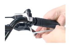
Remove the screws from the bicycle bell and attach the bell to the handlebar tube.
