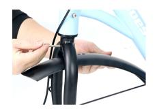
Use a tool to tighten the screws to secure the front fender into the middle of the front fork
