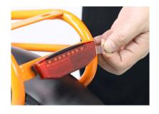
Push the button to switch on the rear lights
