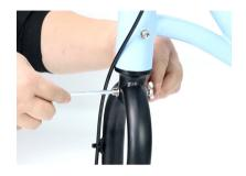
Align the front fender with the hole on the front fork
