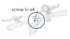
handlebar in the most upward position when tightening the screws.
