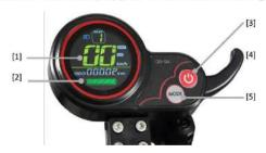
**Gear change.** To change the gear (1=slow, 2=medium, 3=fast), while the scooter is powered ON, press the POWER button to enter gear setting mode. Press MODE to switch between gears. To return to operating mode either press POWER or wait for 2 seconds.
