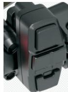
The switch has the following functions: light, turn signal, and horn button. When the light button is pressed, the front and rear deck light will turn on. When the turn signal button is pressed, the front and rear light will turn on and flash. When the horn button is pressed, the horn will sound. When multiple buttons are pressed, the priority for the function from highest to lowest is turn signal, brake, and then light.
