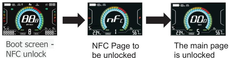
The startup interface will be displayed when the device is powered on. After the communication connection is established, the instrument will enter the NFC page to be unlocked. After swiping the card, the instrument will enter the home page. The meter does the actual display with the information obtained from the controller communication.
