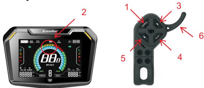
1: Power key 2: NFC Induction region 3: Upper key 4: Function key 5: Down key 6: Acceleration rod
