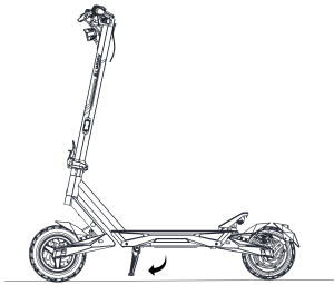
2.After riding the scooter, please release the kickstand and park it in the correct place.
