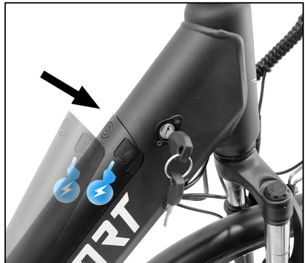
2. Connect the battery socket to the pin and push it up, Turning the key to the "lock" position.
