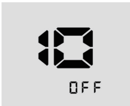
Page "Off": setting the screen timeout; The default screen timeout is 10 minutes.
