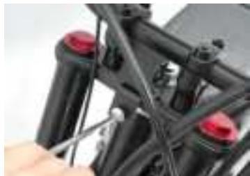
20 Route the front brake hose through the internal cable channel of the license plate bracket
