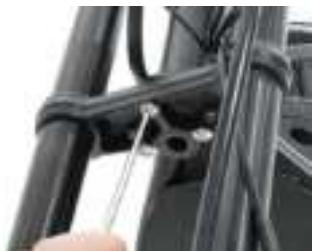
05 Position the mudguard beneath the fork bracket assembly
