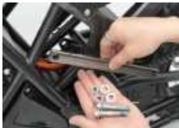
32 Position the shock absorber assembly at the illustrated angle and insert both mounting bolts
