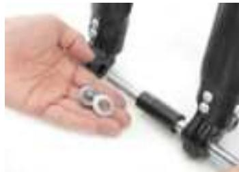
11 Pass the front wheel axle through the shorter spacer on the opposite side, then through the corresponding bearing housing
