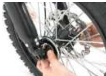
09 Insert the front axle rod through the wheel bearing mounting hole, then pass it through the axle sleeves. Position the longer sleeve on the disc brake side
