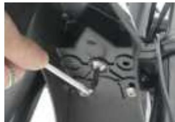
07 Remove the front axle rod from beneath the fork
