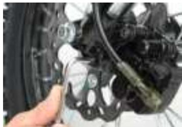
17 Align both the front license plate bracket and headlight mounting bracket screw holes with the corresponding fixing points on the upper fork assembly
