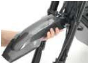
06 Tighten the three mounting screws on the underside of the mudguard
