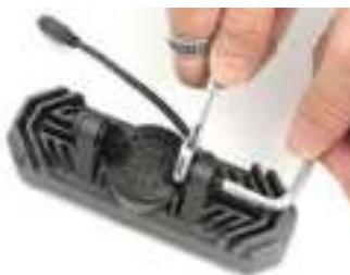
24 Install the headlight onto the mounting bracket and securely tighten the fasteners
