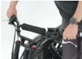
03 Tighten the handlebar clamp screws
