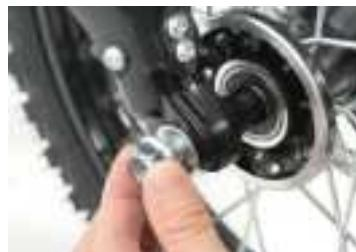
13 Simultaneously tighten both flanged nuts clockwise using the appropriate tool
