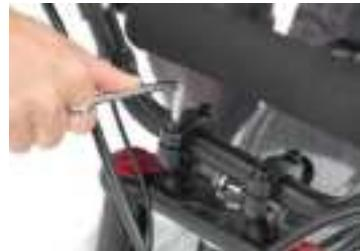
04 Remove the front mudguard mounting screw located below the fork stabilizer bracket
