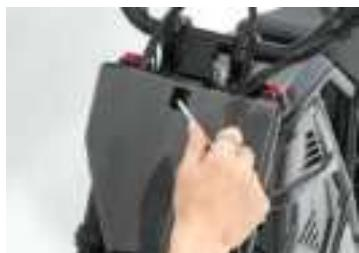
23 Remove the screws and nuts securing the headlight assembly
