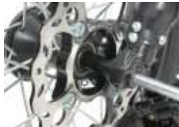
12 Fit the washer into position, then install the flange nut
