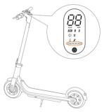
1. Power on the X8 and check the power level indicator. Charge the X8 if the battery level is low.
