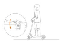
4.Slow down by releasing the throttle; and brake by squeezing the brake lever.
