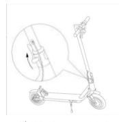
Using hex wrench in the packing box to tighten the screws on handle bar
