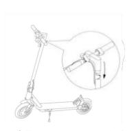
4). Testing the power switch after finish assembling
