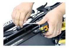
Press down on the folding lever 05 and lift up the upright lever
