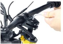
Remove the instrument bracket 11 from the bag and install the rubber pad
