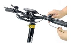
While pressing the limit button, 16 pull the pole upwards until it reaches the appropriate position
