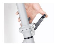
Ensure that the folding buckle is securely locked, which is a prerequisite for safe driving
