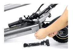
Align the screw holes and insert the screws
