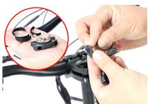
Place the rubber pad into the bracket of the instrument panel
