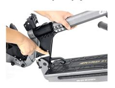
After the pole is fully extended, snap the safety buckle into place
