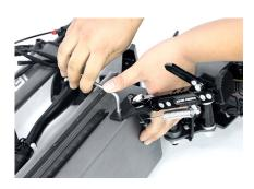
Press down on the folding lever and lift up the upright lever
