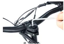
Fix the instrument panel in the middle position of the handle and tighten the screws
