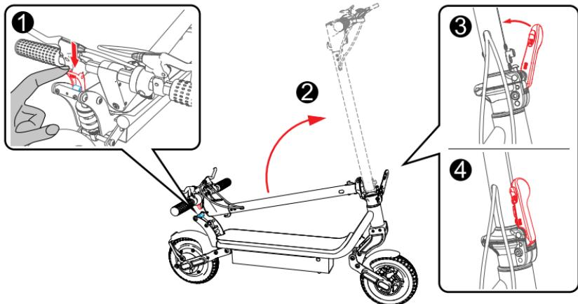
**EN** Press the folding buckle to release the handlebar from the rear fender and lift the stem to the riding position. Then close the folding latch until you hear a click.
