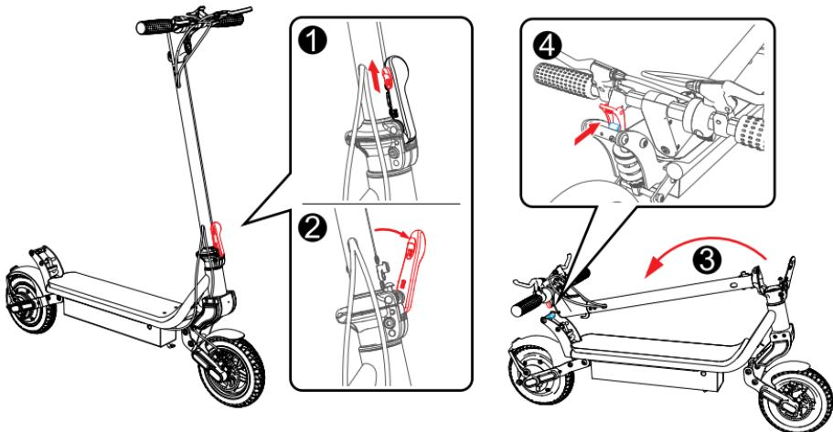
**EN** Turn the scooter off, open the folding latch, fold down the stem so that the hook on the rear fender catches the folding buckle on the handlebar.
