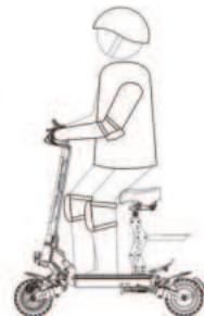
4. Release the accelerator and the speed will slowly drop to a stop; If you need to decelerate quickly, slowly squeeze the brake lever while releasing the accelerator.
