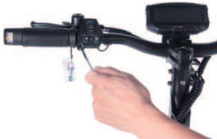
7. Adjust the throttle lever to the desired position using a S4 wrench and secure it firmly.
