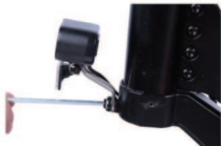
5.To install the rear fender: Align the fender with the screw holes on both sides of the rear wheel and securely fasten all four screws.
