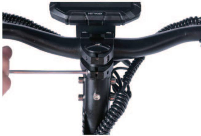
4.Using a S5 wrench, remove the screw from the frame, install the headlight assembly, and securely tighten its mounting screw.
