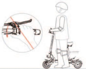
⚠ Do not press the accelerator when you're walking alongside the scooter.
