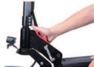
3.Using a S4 wrench, first remove the top clamp cover from the steering column. Align the handlebar's center clamp holes with the column, tighten the side screws, then reinstall and tighten the clamp cover screws.
