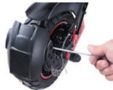
6.Adjust the multi-function switch to the desired position using a S4 wrench and secure it in place.
