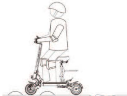
⚠ Keep your speed between 5-10 km/h when you ride through speed bumps, elevator door stills, bumpy roads or other uneven surfaces. Slightly bend your knee to better adjust mentioned surfaces.
