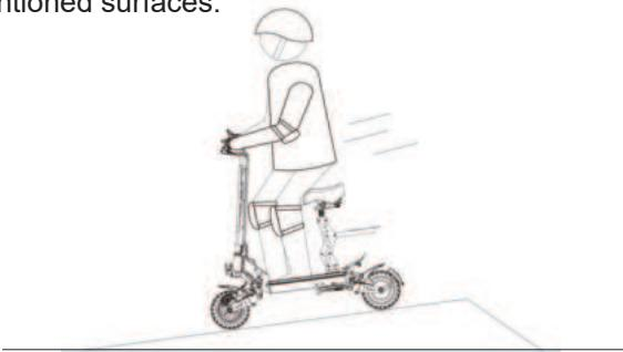
⚠ Do not accelerate when going downhill, and brake in time to slow down. When encountering a steep incline, you need to step off the scooter and push, do not risk riding up.
